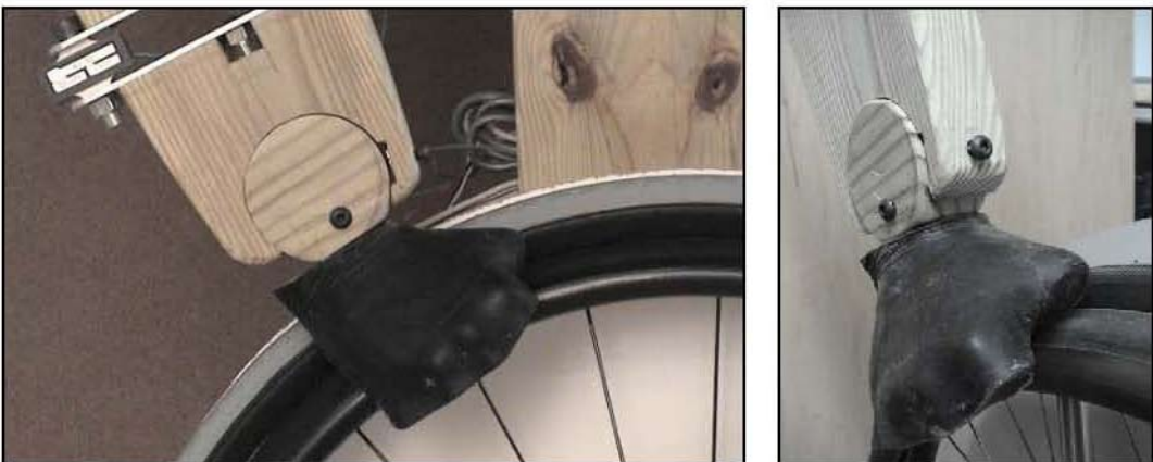
Figure 3. The hand interface of the impact fixture used in this study was molded to the shape of a human hand postured similar to that seen just prior to impact with the handrim.
