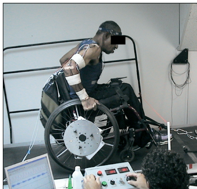
Fig 2. The experimental setup used in this study included a research treadmill, a surface electromyographic measurement system, and an instrumented wheel.
