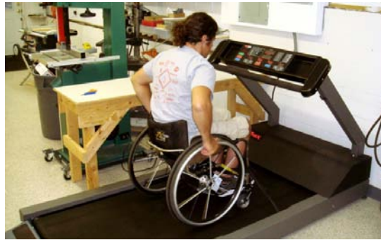
Figure 1: The treadmill has a large propulsion deck, a ramp for boarding, and a dynamic safety system.
