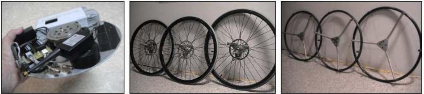
Figure 1: The propulsometer contains a separate instrumentation module that is removable and easily mounted onto any standard wheel size, allowing the propulsometer size to match that typically used by the test subject.
