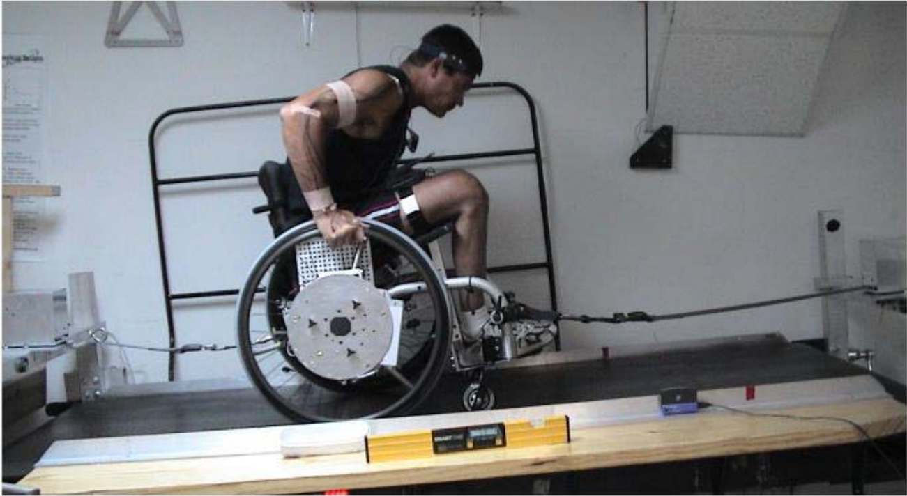
Figure 2. A dynamic wheelchair constraint system has been developed to allow safe wheelchair propulsion testing on a multi-grade treadmill. Treadmill propulsion is an actual rather than simulated propulsion environment, resulting in accurate inertial, resistance and stability performance for any particular individual wheelchair user.
