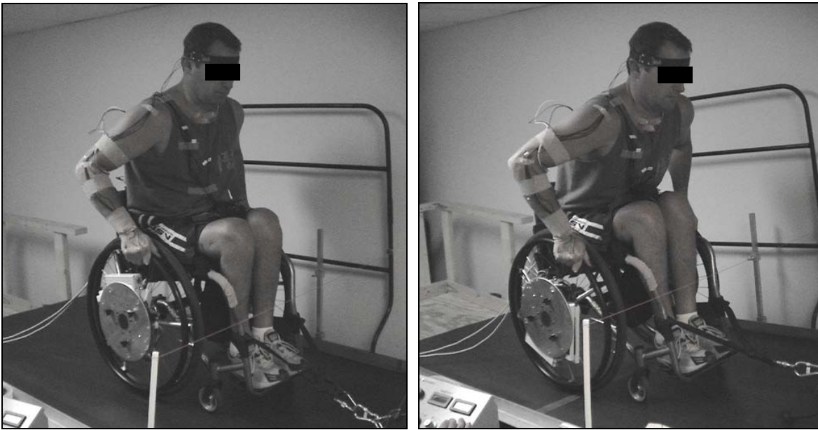
Figure 2. The experimental setup included the subject pushing his/her own wheelchair on a research treadmill. The instrumented test wheels allow the forces and moments applied to the handrim to be measured. Motion capture markers were used to track the location of the wheel and 3 rd MP joint of the hand.
