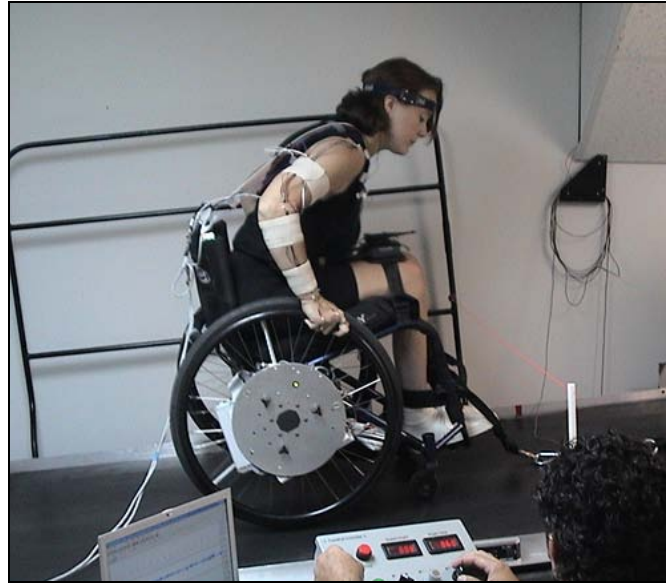
Figure 2. The experimental setup used in this study included a research treadmill, an instrumented wheel and a motion-capture system.
