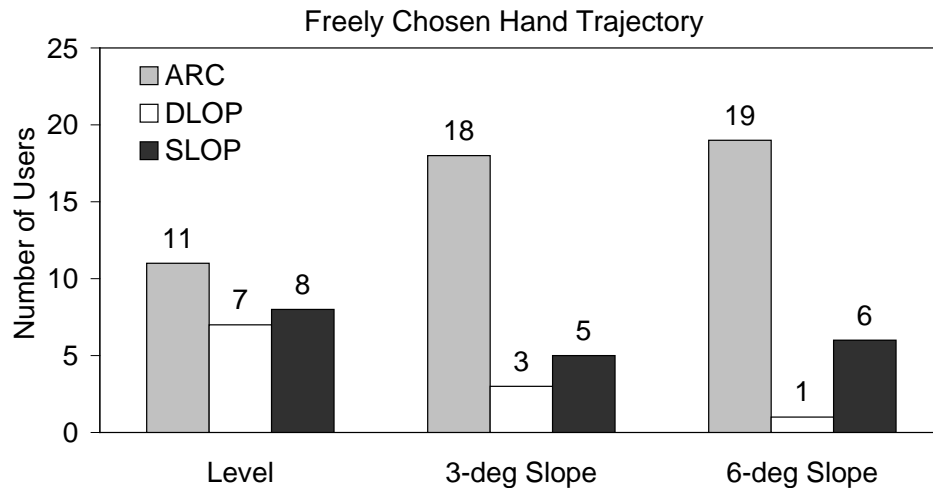
Figure 3. The freely chosen recovery patterns were fairly balanced for level propulsion but the ARC pattern became the most popular for pushing uphill.
